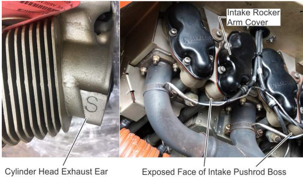
Figure 3. Cylinder Head Indicates Prior Compliance, Stamped with Letter “S”
