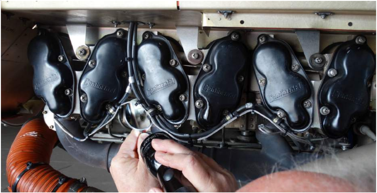
Figure 5. Cylinder Head Inspection Area, typical aircraft installation
