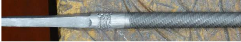
Figure 7. Round Nickolson Bastard Cut File or equivalent, 1/4” diameter
