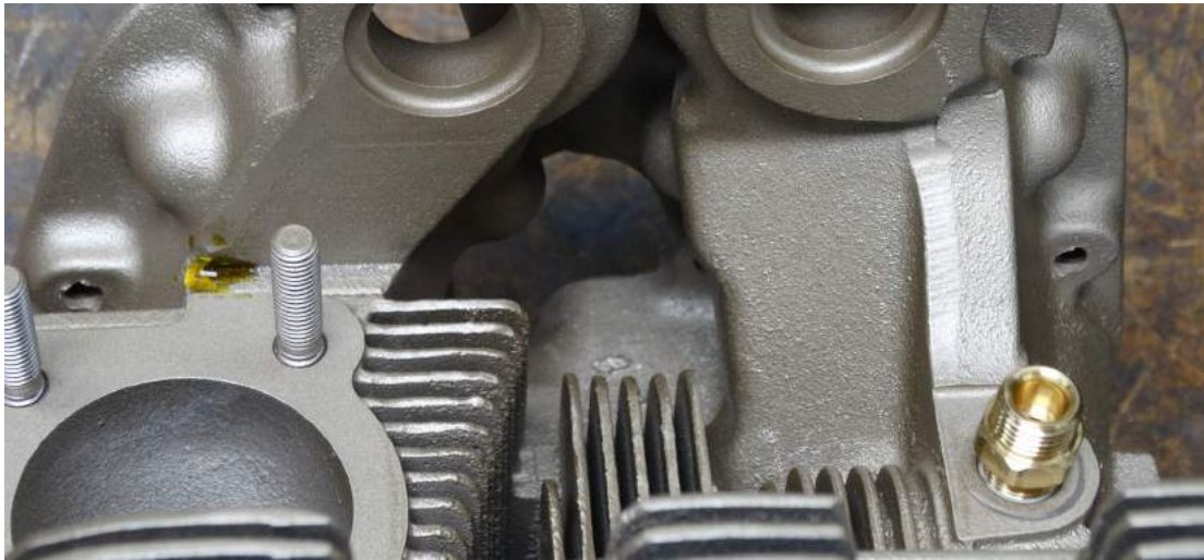
Figure 8. Cylinder Head, Alodine Application
